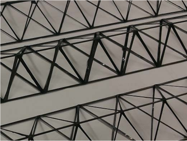
pre-series carbon-fiber ladders (GSI)
