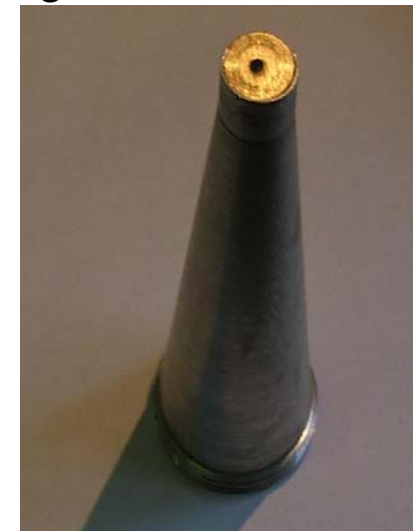
Pin-hole EUV camera with thin ( 1,5 \mu\text{m} ) \text{Be} + \text{BeD}_2 composite optical filter
