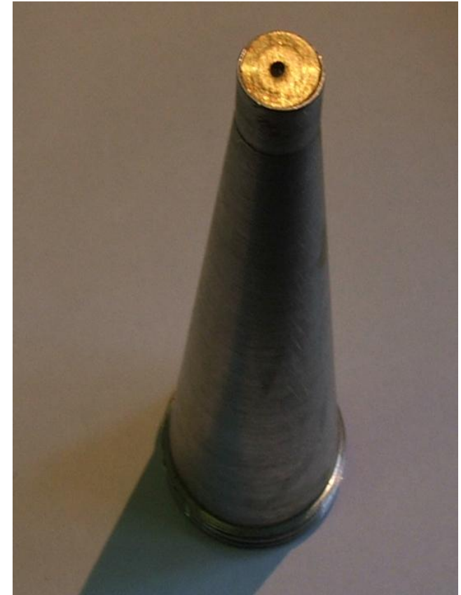
↑ Photograph of pin hole camera with thin (0.5 micron) ( \text{Be}+\text{BeH}_2 ) x-ray filters
