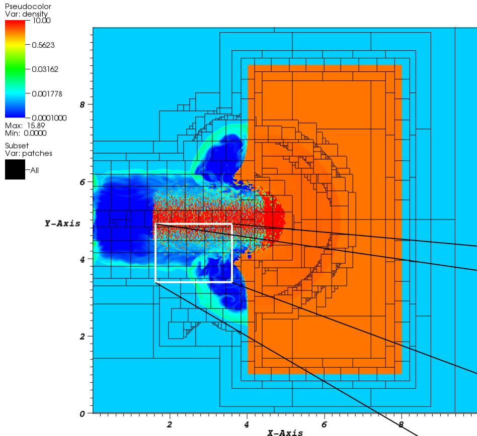
Refinement is applied in zones of interest (interfaces, high gradients of parameters) while the rest of domain is resolved on a coarse mesh
