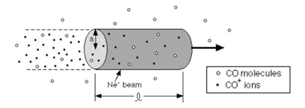
Scattering ionization (depends on cross section σ<sub>ion</sub>)
