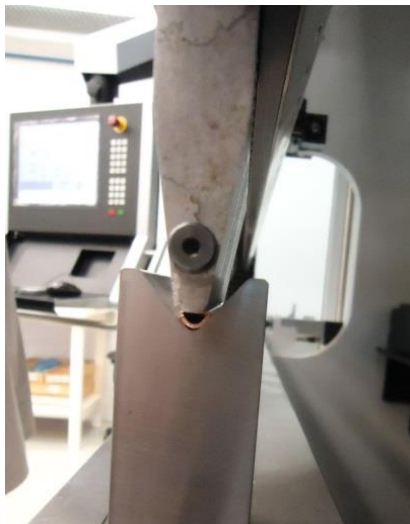
Cooling tube forming starting from \varnothing 6.35 \times 1 \text{ mm}
