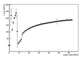
Discontinuity (probably) due to which clock edge is used for calculation (i.e. the first one after a falling edge).
