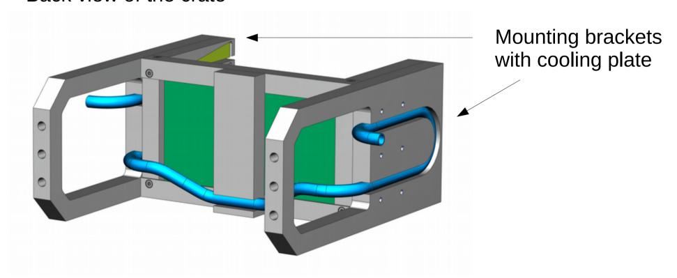
Can a single aluminium pipe can be used to cool several crates (avoid joints)?
