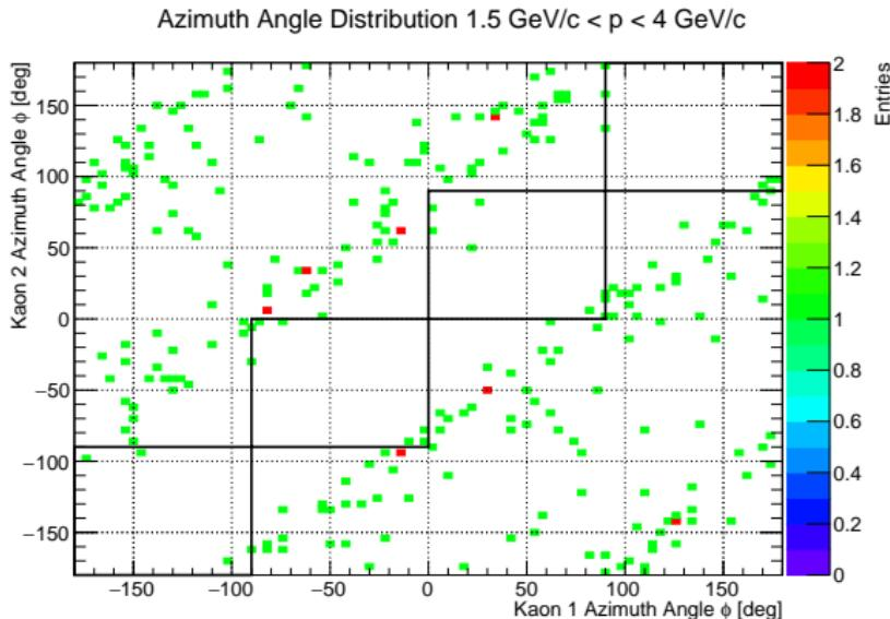
Many events with  $K^+/K^-$  traversing through two different radiator quadrants  $\rightarrow$  less pile-up
