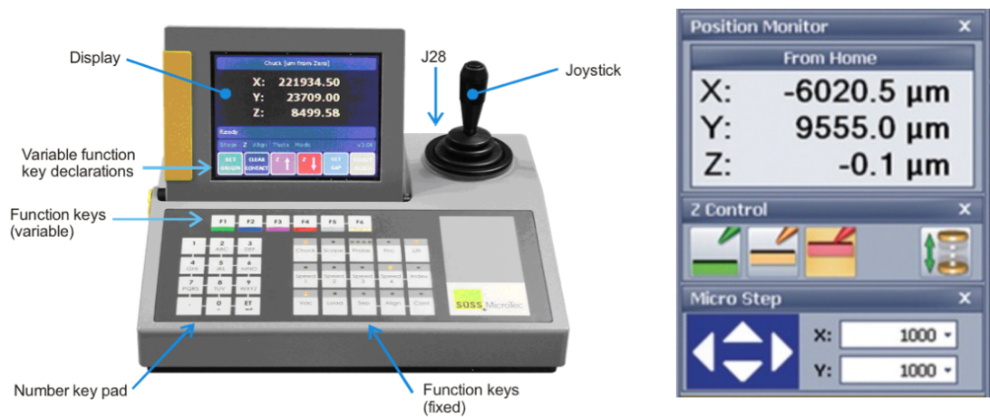
Figure 4.5: General view of the Süss Expert Control Panel (left); Chuck controls of the PC based operating system (right).
