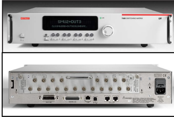
Figure 5.10: Front and rear views of the Keithley 708B mainframe with the switching card 7072-HV installed [101].
