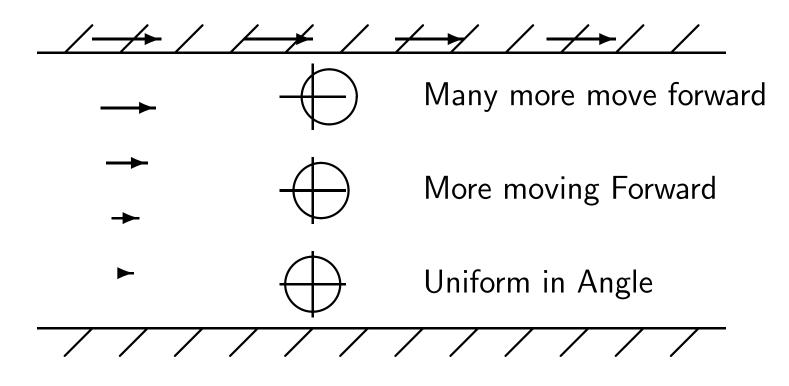
Fluid in between has varying velocity
