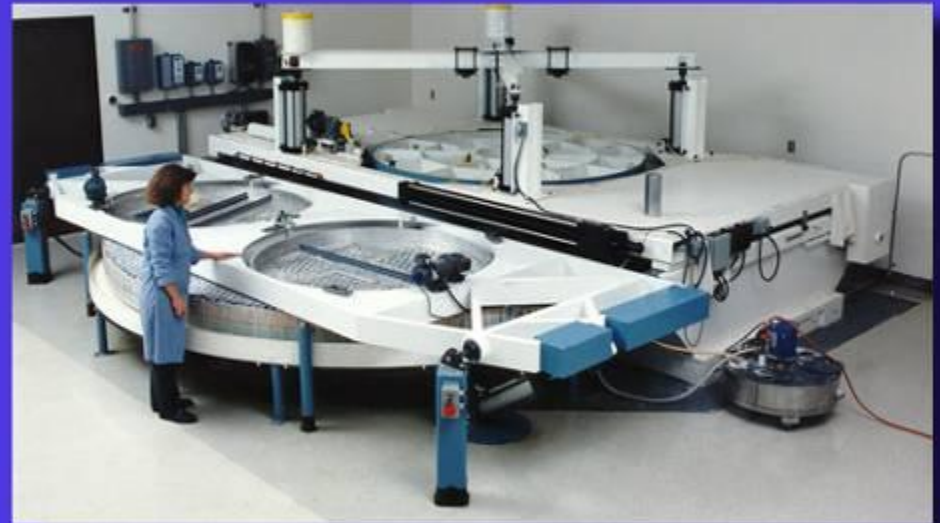
14 Foot (4.3 Meter) Diameter Polishing Machine
