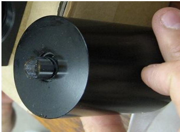
10mm \phi quartz + MCP-PMT
