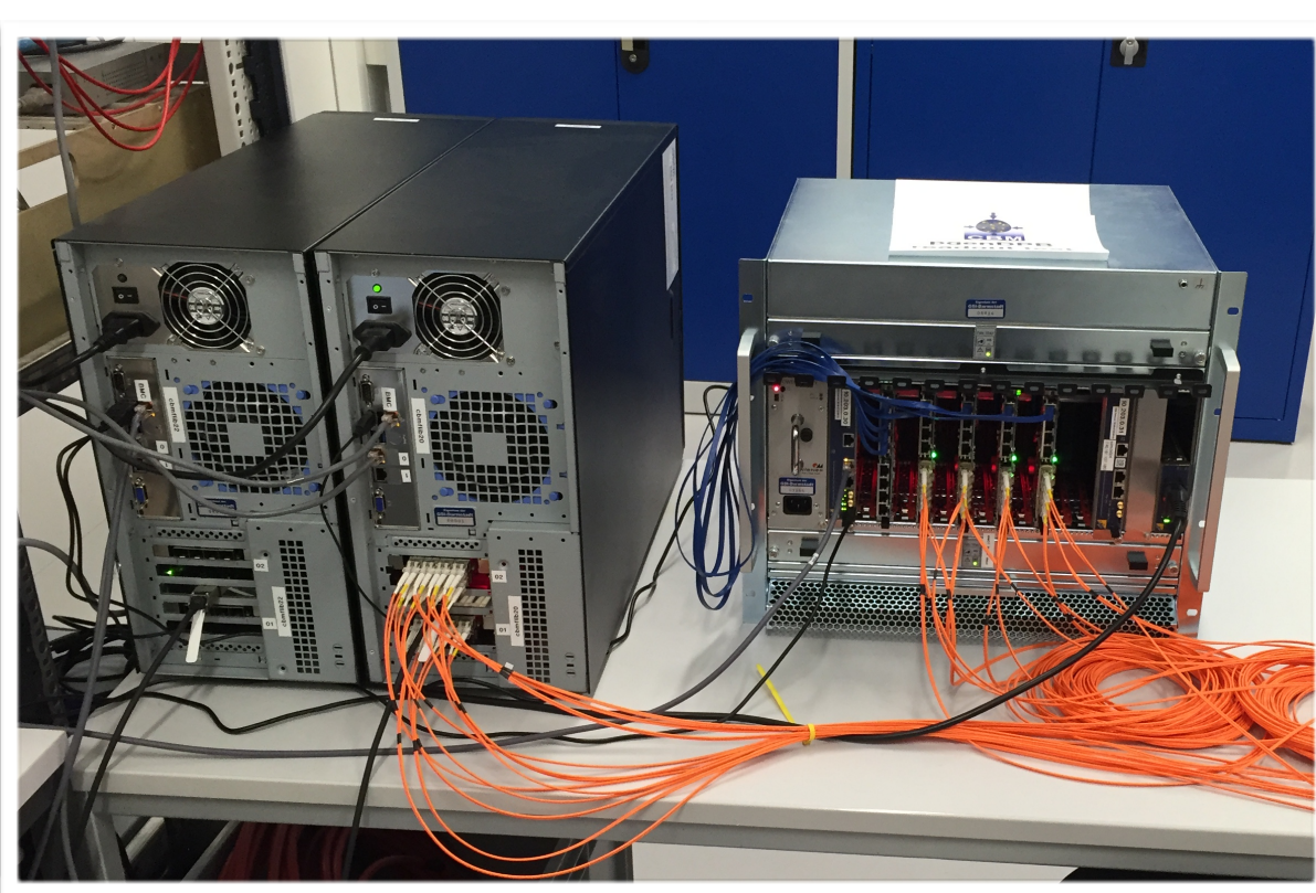
Setup with DPB layer in MTCA crate
