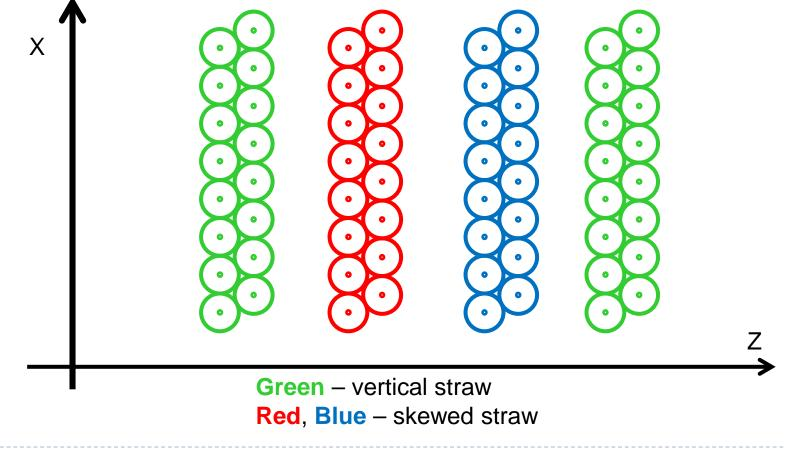
Data structure for storing the geometry of the detector
