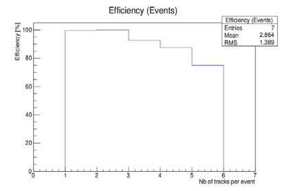
Algorithm efficiency as function of number of good tracks in events (good=min 13 layers with hit)
