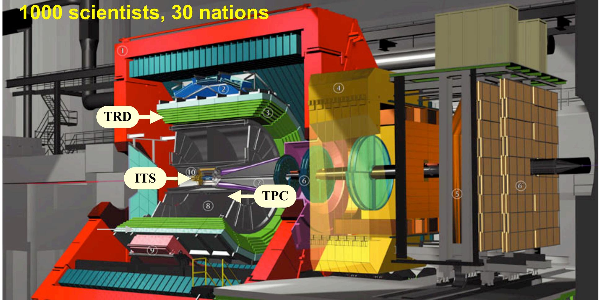
**ITS:** measures secondary vertex, open heavy-flavor, c and b
