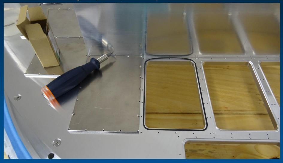
O-rings & max torque screwdriver
