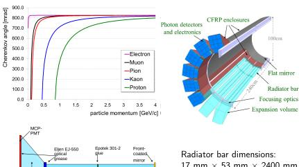
Radiator bar dimensions:  $17 \text{ mm} \times 53 \text{ mm} \times 2400 \text{ mm}$ 48 radiator bars in 16 sectors
