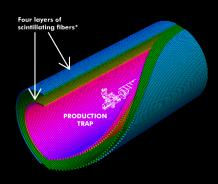
fiber diameter has been scaled up four times to allow visualization
