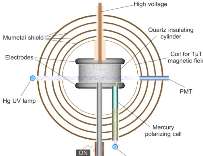
Mercury co-magnetometer (1998)
