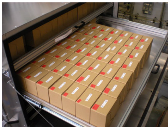
13/05/2016 Storing of 160 PMTs in the top compartment N_2 flow : 15 l/h
