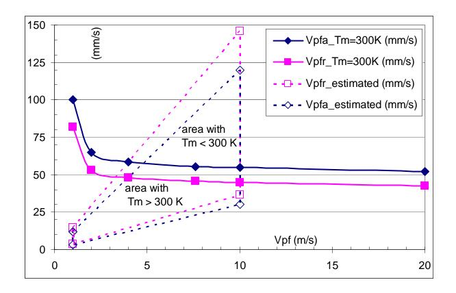
For half of the estimated volume ( $V_{pf}$ ,  $V_{pfa}$ ,  $V_{pfr}$ ), we have  $T_m > 300 \text{ K}$  which would require the use of a dump resistor
