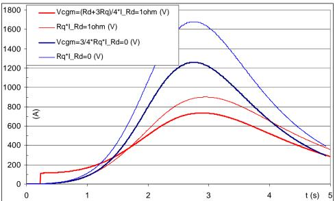
In that particular case, using  $R_d$ = 1  $\Omega$  enables to reduce  $T_m$  from 458 to 351 K and  $V_{cgm}$  from 1260 to 736 V.
