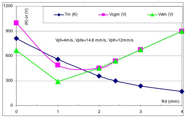
In that example  $R_d = 2.4$  ohm gives  $T_m = 300 \text{ K}$ For each  $(V_{pf}, V_{pfa}, V_{pfr})$  triplet, it is possible to find  $R_d$  so that  $T_m = 300 \text{ K}$
