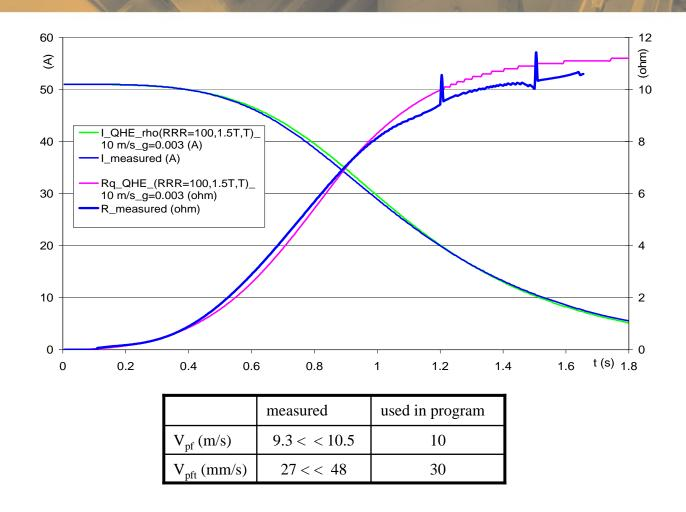
The quench program was validated on a 6 kJ dipole when using measured quench propagation velocities
