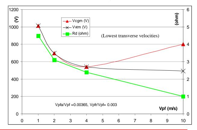
For the lowest transverse propagation velocities, it is possible to have:  $T_m = 300 \ K \ and \ V_{cgm} < 1000 \ V$
