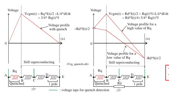
V<sub>cgm</sub> will be see at point A or B V<sub>vtm</sub> will be seen at point A or C
