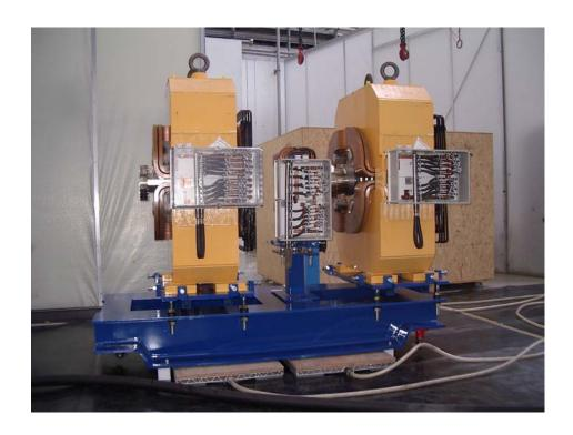
Quadrupol duplet with vertical steering magnet for the Heidelberg Therapy Project (HIT)
