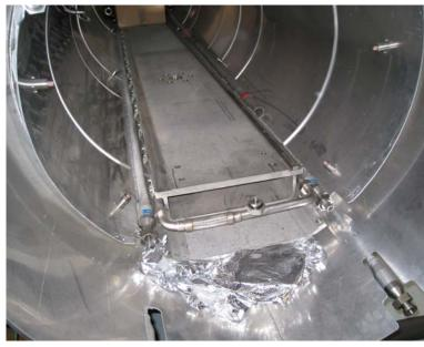
The link to the cryostat (shield and vacuum vessel) is done by composite tubes.
