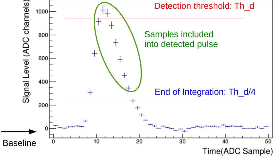
Pulses of proper shape will be properly detected close to the threshold
