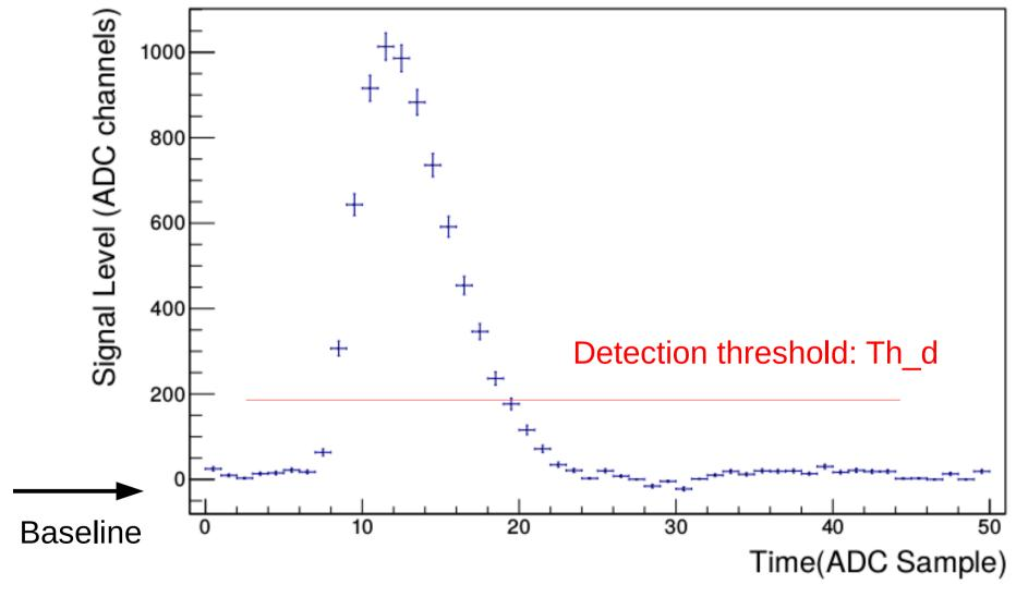
Straight-forward pulse detection: Threshold crossing
