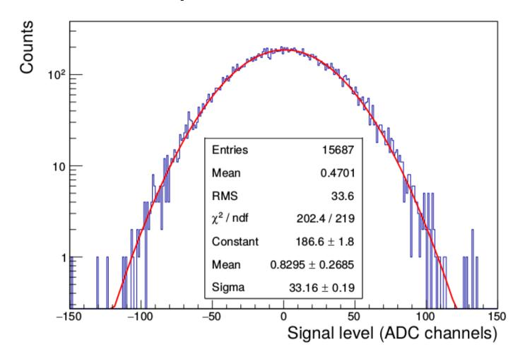
Straight-forward pulse detection: With threshold of **100** we should expect rate of 100 kHz
