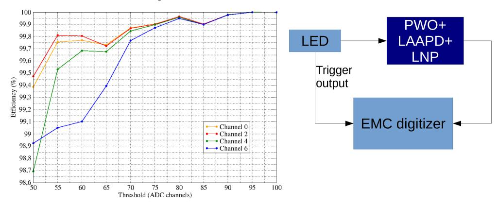
For pulses with amplitude well above the threshold efficiency does not suffer significantly from reduced threshold:
