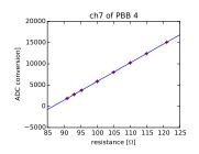
$$R_{k} \cdot \underbrace{I_{k} \cdot G_{k} \cdot C}_{m_{k}} + \underbrace{U_{\text{off}} \cdot C}_{n} = N_{k}$$
