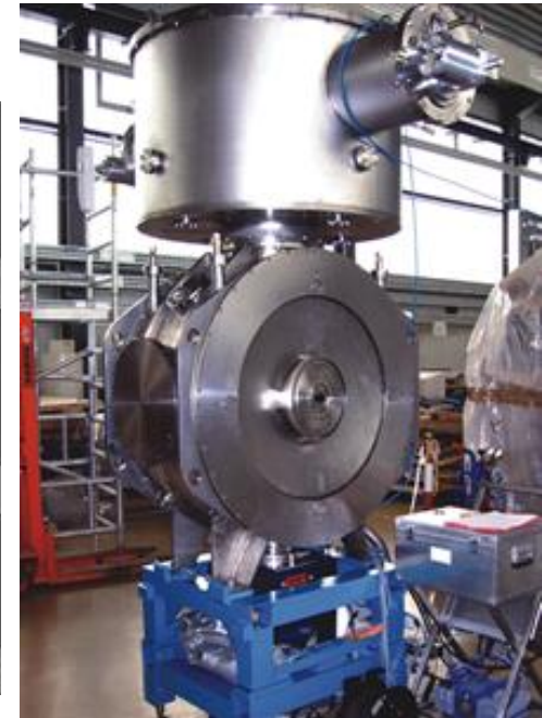
9 T superconducting magnet
