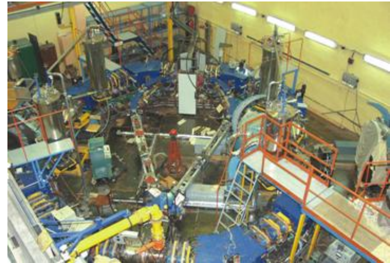
VEPP-2000 - the first collider with round beam option
