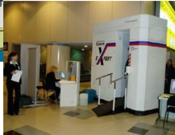
Anti-terror X-ray system in airport
