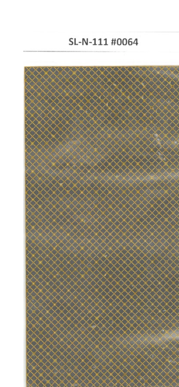
2 shielding layers and spacers
