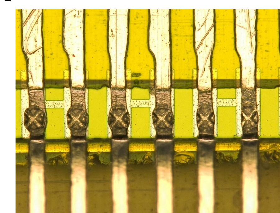
aluminum traces, TAB-bonded to bond pads of a silicon sensor
