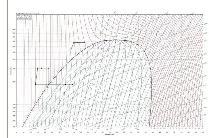
TRAXI XL provides liquid CO<sub>2</sub> in the temperature range from -40°C to 5°C at the bi-phase boundary. The diagram shows two possible **thermodynamical cyles**, the latent heat will be used in the heat exchanger for cooling up to 50% vapor quality.
