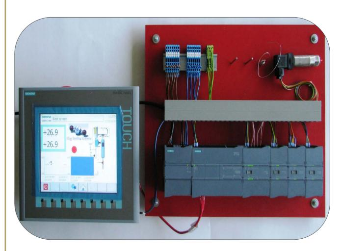
The cooling plant is fully controlled by a standard **PLC Siemens S1200**.
