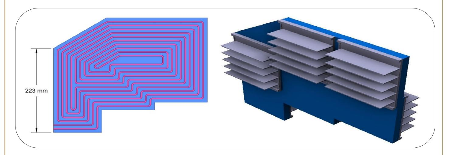
Traci XL will be used to test the cooling efficiency of a 1 kW quarter station cooling demonstrator. **Heat exchangers** (in blue) take the thermal load form the front-end electronics. The left side figure shows the channels for the liquid CO<sub>2</sub> flow in the heat exchanger; the right side figure show the cooling plate with shelves for the front end boards attached.
