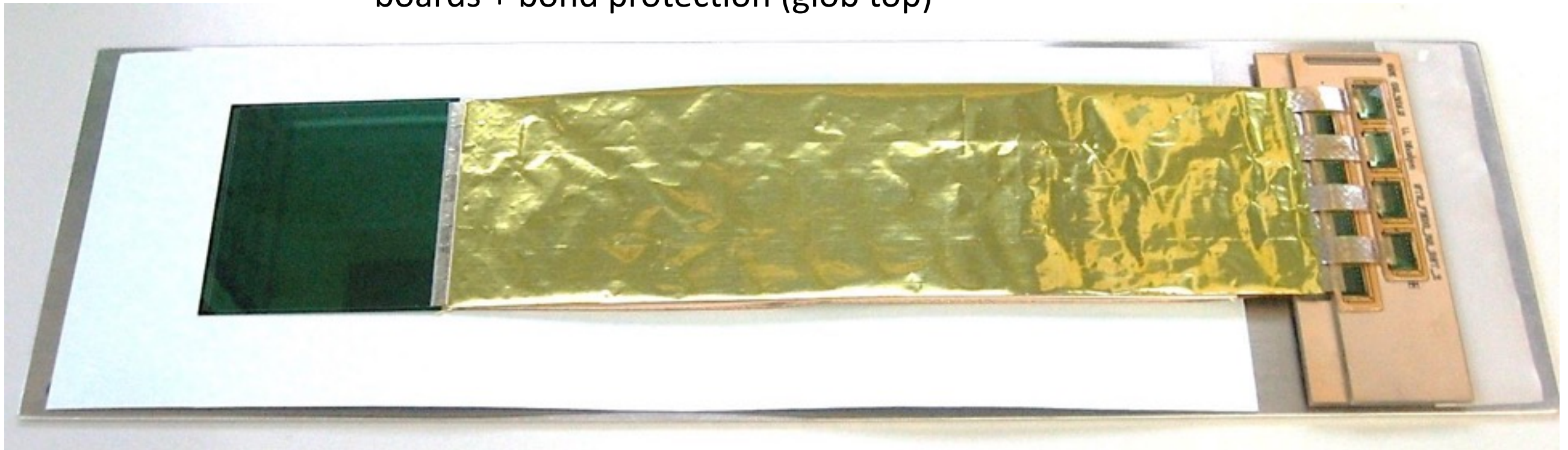
2. Wire bonding ASICs to front-end boards + bond protection (glob top)
