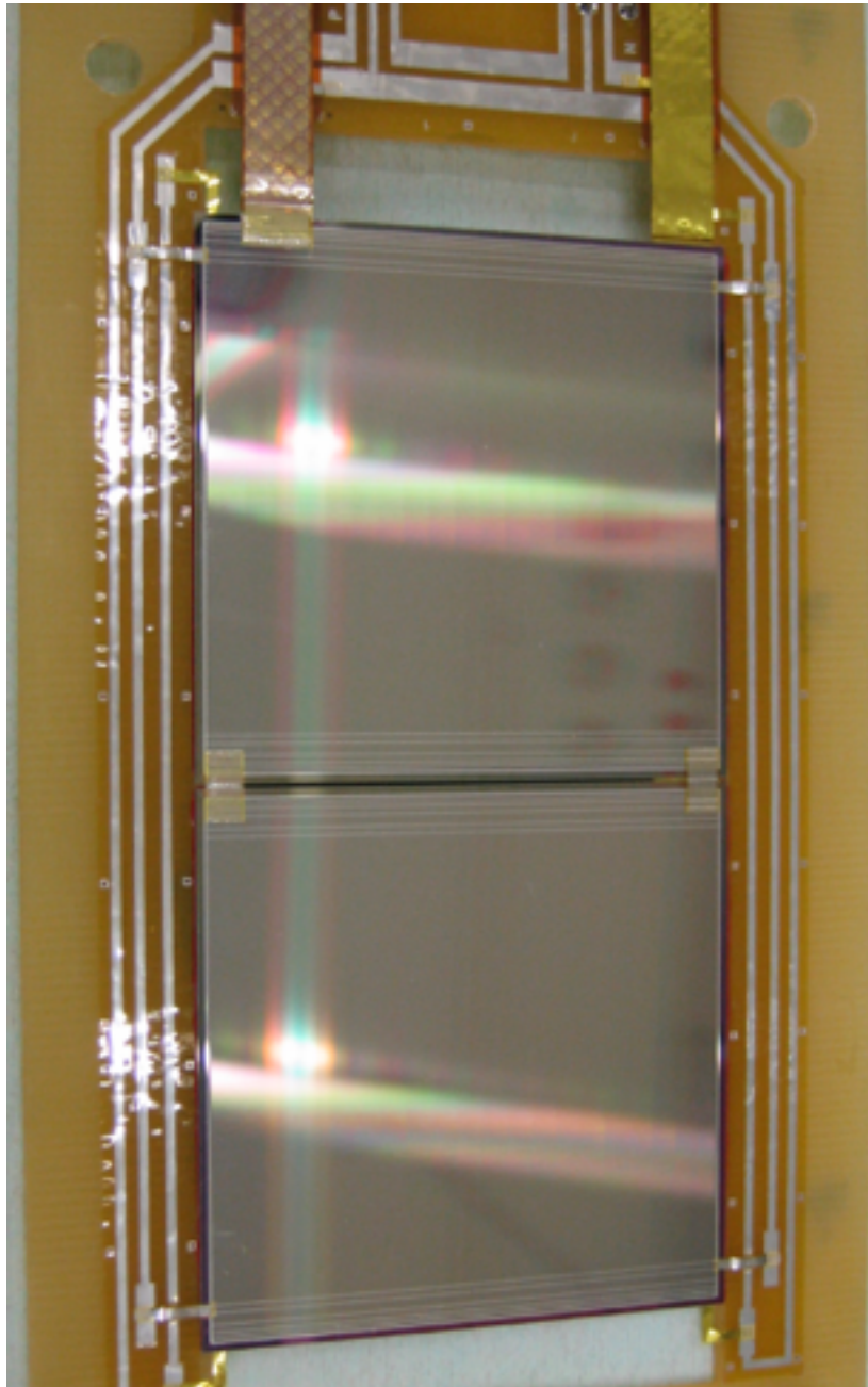
two daisy-chained sensors with 6 \times 6 \text{ cm}^2 size each
