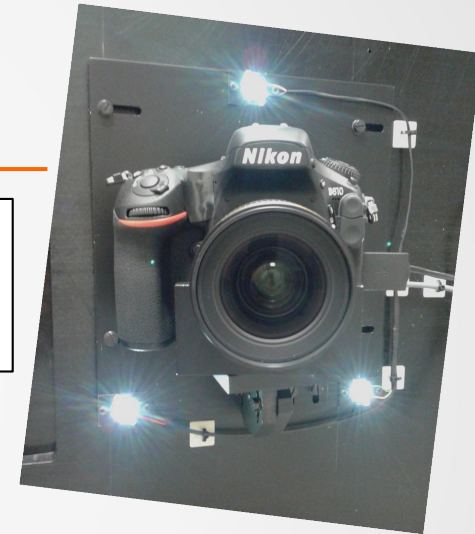
CLAM camera surrounded by 3 LEDs
