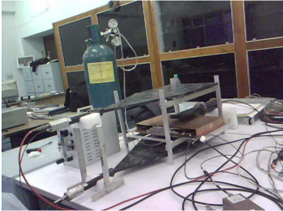
Figure 4.11. GEM detector under test with cosmic MIP's at VECC.
