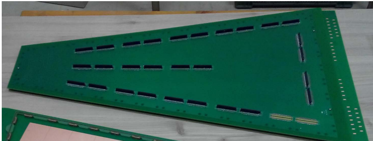
Readout PCB outer side with FEB connectors
