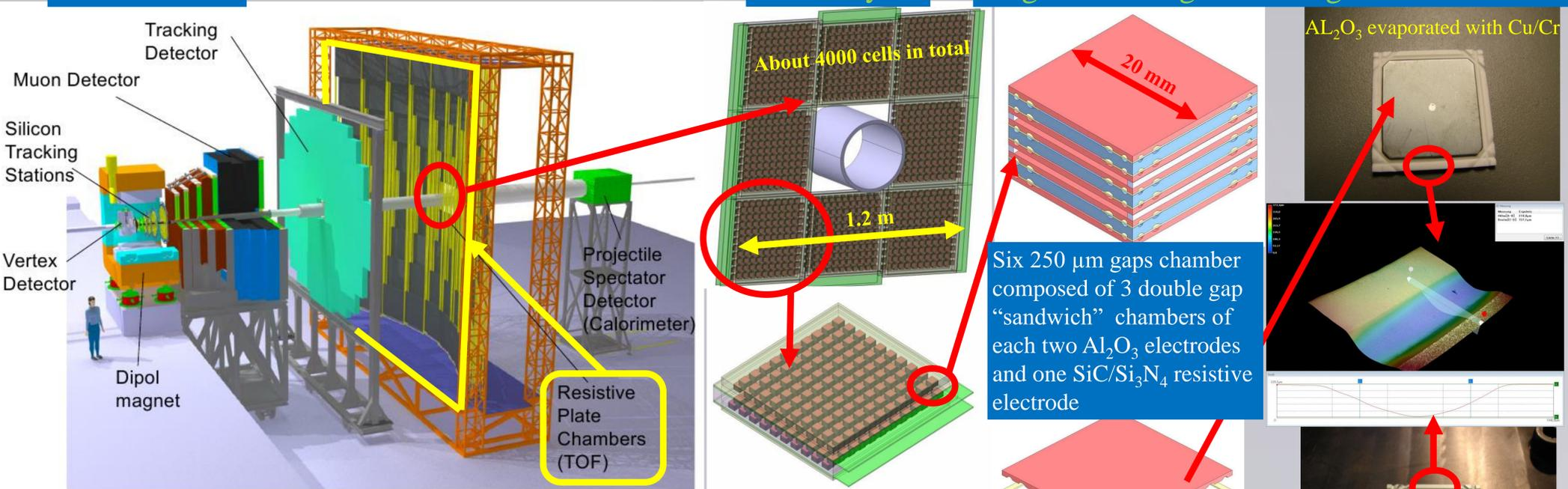
The present work aims at the development of the Beam Fragmentation  $T_0$  Counter (BFTC) of the CBM experiment. This detector will be located at the forward region around the beam pipe, where the particle flux is expected to be as high as  $2 \times 10^5 \text{ cm}^{-2} \text{ s}^{-1}$ .
