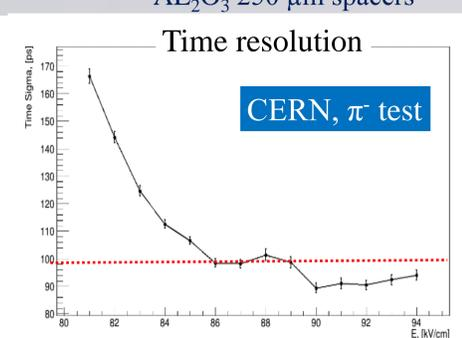
Bulk resistivity  $5 \times 10^8 \text{ Ohm} \cdot \text{cm}$  is too low to operate stably at HV plateau;  $2 \times 10^{10} \text{ Ohm} \cdot \text{cm}$  is too high to operate at rates higher than  $100 \text{ kHz/cm}^2$ . Efficiency ( $\sim 96-98\%$ ) and time resolution ( $\sim 80-90 \text{ ps}$ ) are consistent with expectation. MAXIM 3760 preamplifier was used, for comparison with ALICE R&D data.
