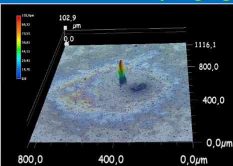
The 90%  $\text{C}_2\text{H}_2\text{F}_4$ /10%  $\text{SF}_6$  or 95%  $\text{C}_2\text{H}_2\text{F}_4$ /5%  $\text{SF}_6$  binary gas mixtures were used, since the formerly used iso-butane was found to be responsible for whisker formation (photo).
