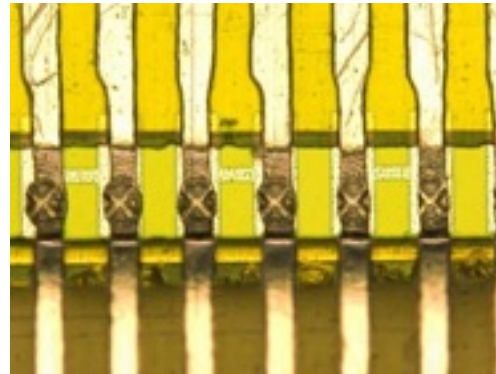
TAB bonding of microcables to ASICs and sensors
