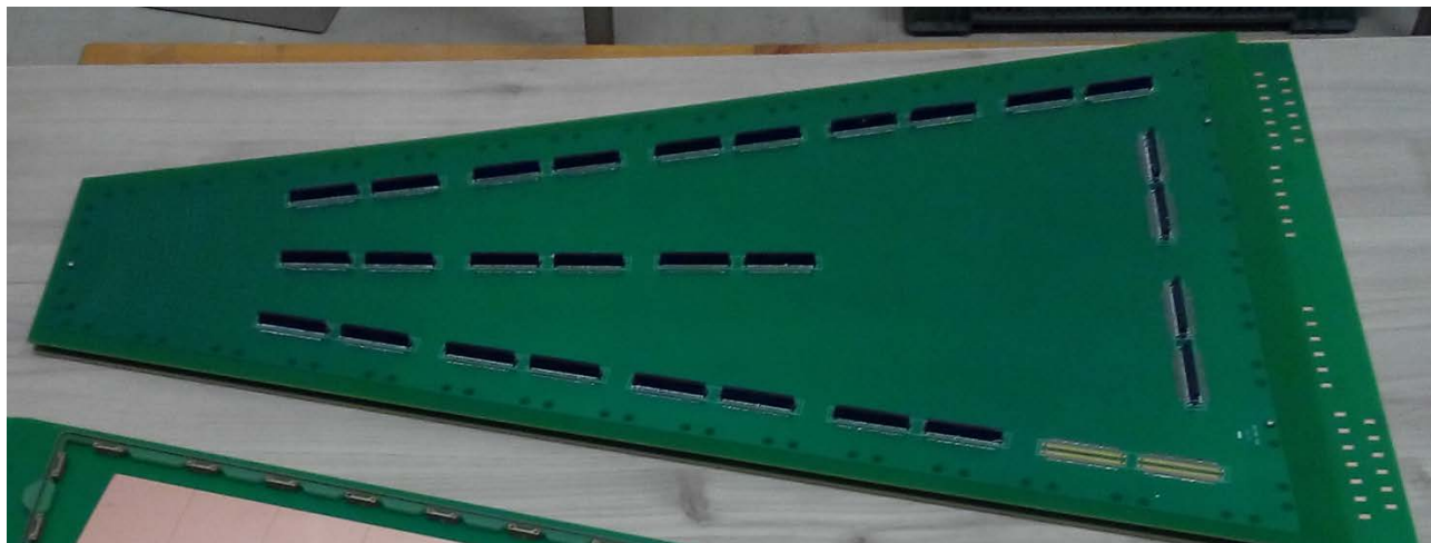
Readout PCB (8-layer) outer side with 15 FEB connections (nXYTER)
