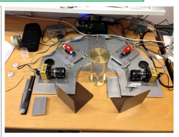
Integrated measurement level with 2 lasers and 2 LS-cameras being aligned in a desktop setup using 5 fishing lines.
