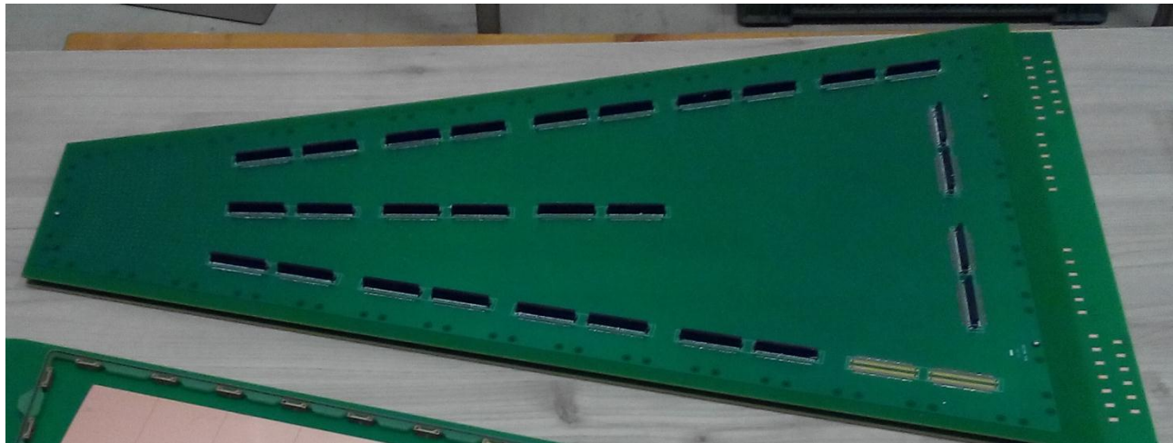
Readout PCB outer side with FEB connectors
