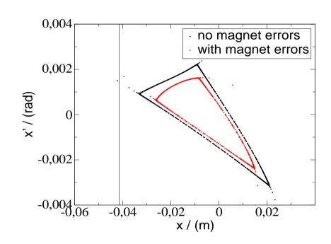
Beam loss of  $\sim 10~\%$  distributed around the ring, i.e. not at ES septum.
