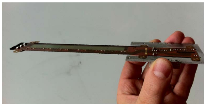
Figure 24: Picture of a prototype Silicon ladder developed within the PLUME project.
