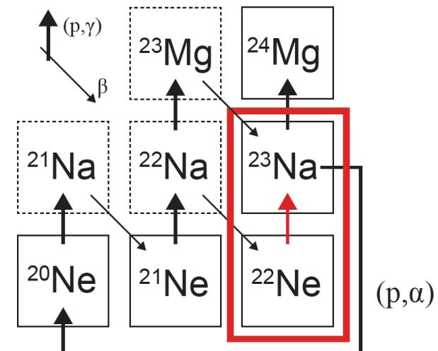
$^{22}\text{Ne}(\text{p},\gamma)^{23}\text{Na}$  is the most uncertain reaction in the NeNa cycle
