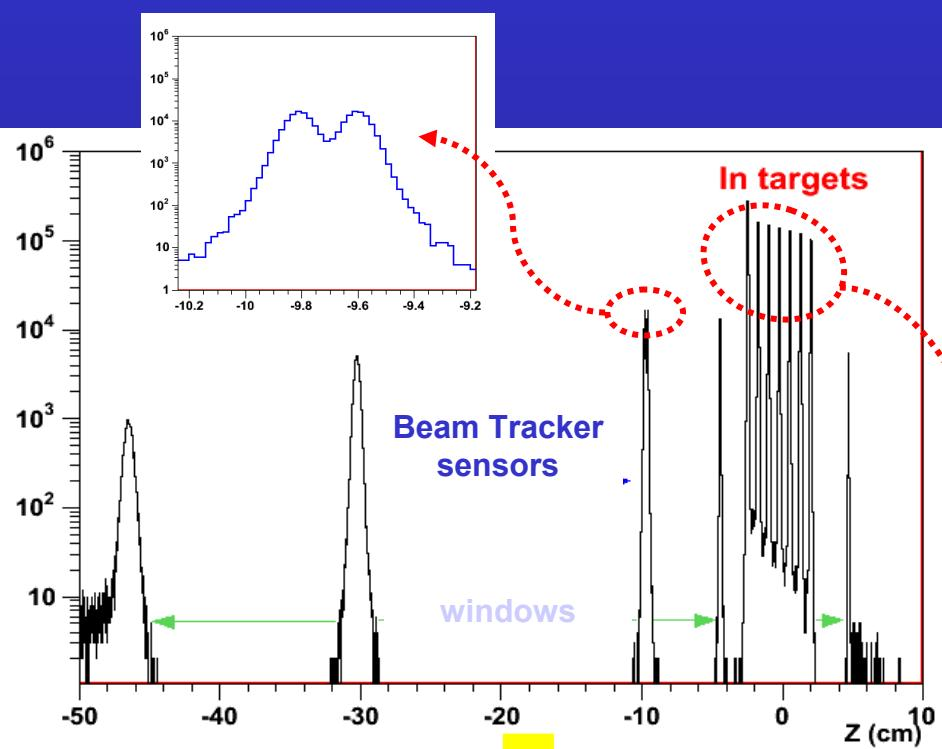
$\sigma_z \sim 200 \mu\text{m}$  along the beam direction
