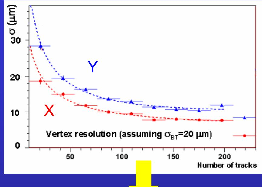
Resolution  $\sim 10 - 20 \mu\text{m}$  in the transverse plane
