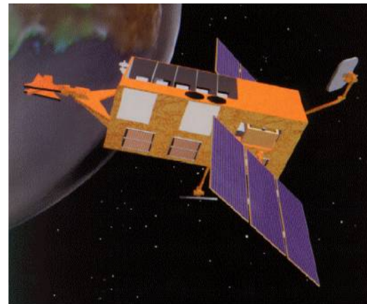
Rossi X-ray Timing Explorer 1995 2 – 250 KeV, 1 degree Large collecting power High time resolution
