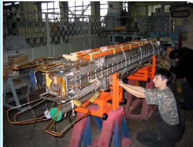
Figure 17 SIS100 curved magnet assembled without vacuum chamber.
