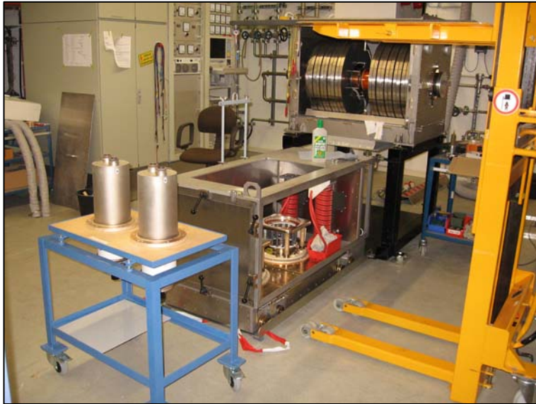
Short pulse (500 \mu\text{s} ), high power bunch compressor developed at GSI
