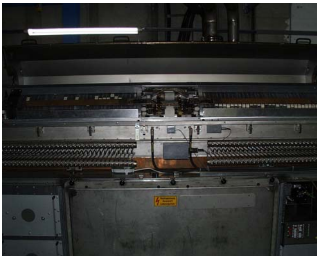
SIS18 ferrit loaded accel. cavity
