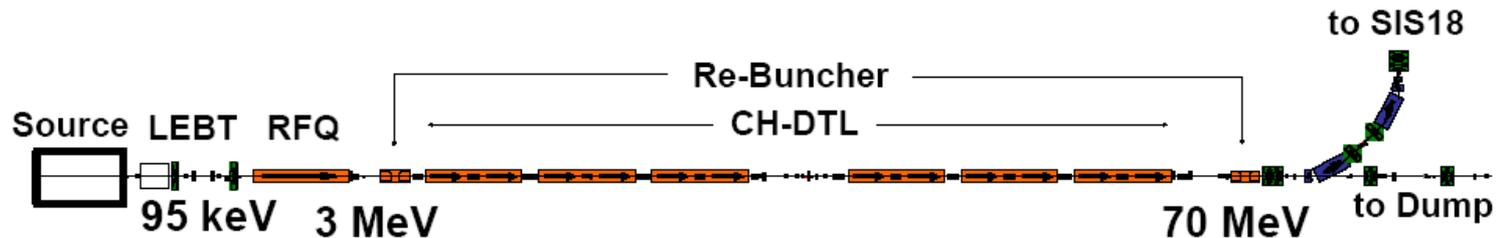
Conceptual layout of the proton linac of FAIR comprising a proton source, a RFQ, and a Drift Tube Linac (DTL) based on 12 CH-cavities.
