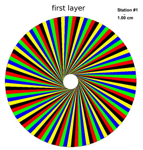
strip pitch: 300µm at the inner radius strips tilted by 60° to radial strips at the inner radius
