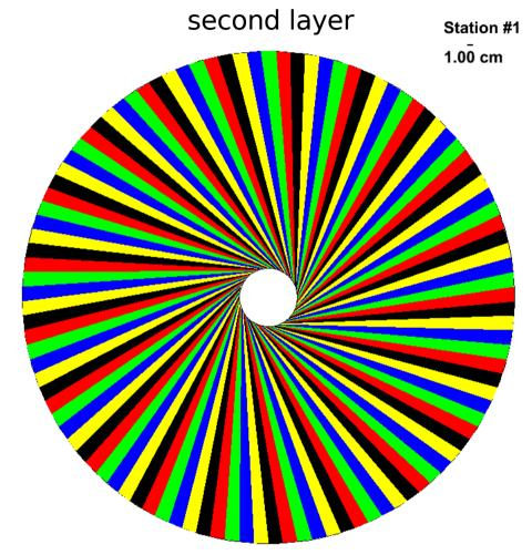
strip pitch: 300µm at the inner radius strips tilted by -60° to radial strips at the inner radius 8 ~1571 strips per station
