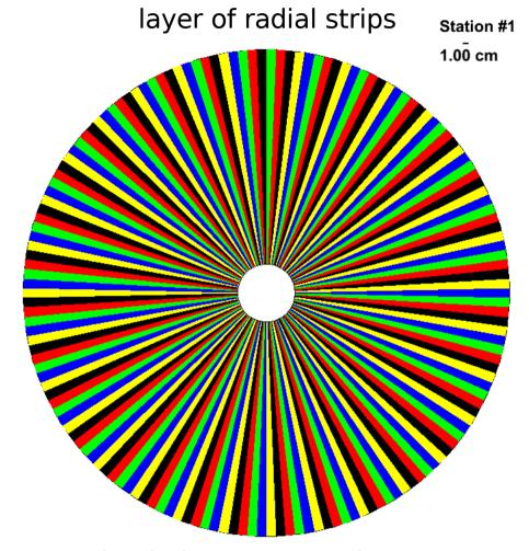
strip pitch: 200µm at the inner radius ~1048 strips per station
