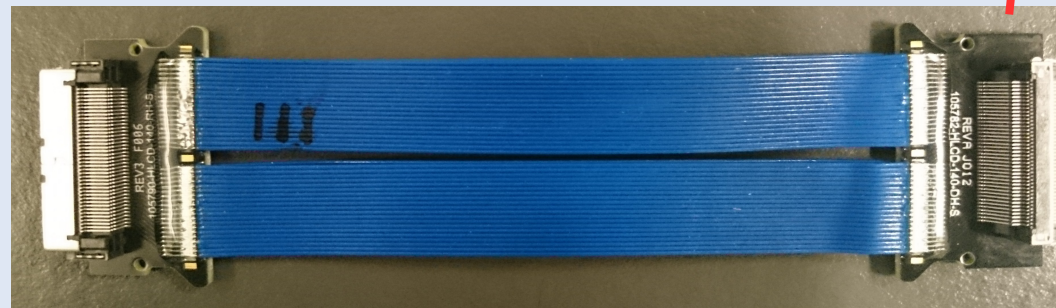
Samtec HLCD microcoax cable mates with LHSM plug
