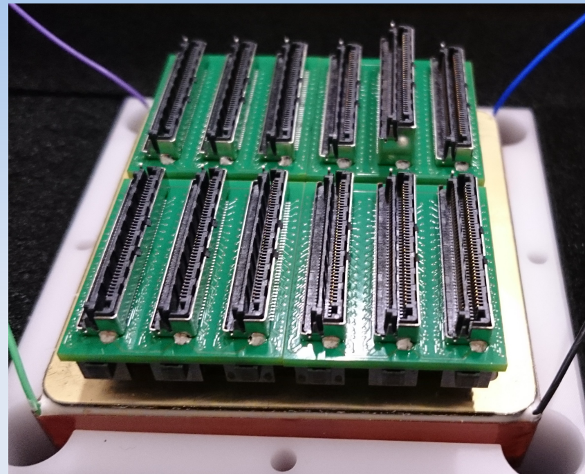
Samtec LSHM plug 2 rows á 40 pins Part: LSHM-140-02.5-L-DV-A-S-TR
