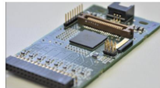
(b) The PaDiWa front-end boards have connectors to directly connect them with the photon sensors.
