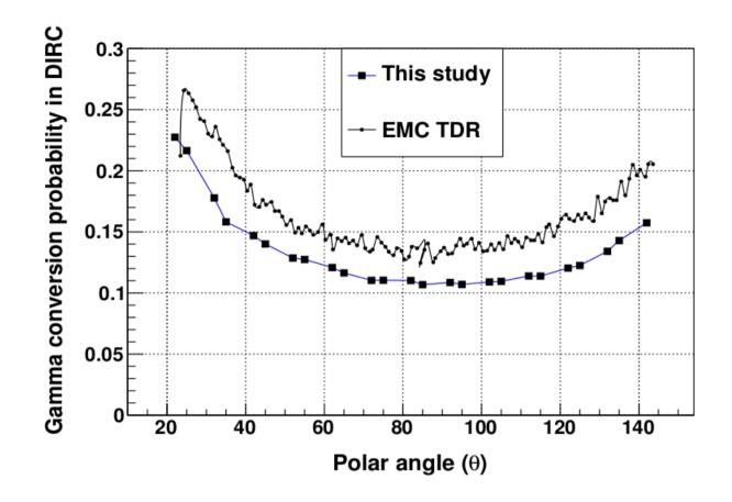
The variation of gamma conversion probability with the polar angle is compared with that in EMC TDR. Though the shape of the both graphs are more or less same, there is a constant mismatch throughout the range of the polar angle.
