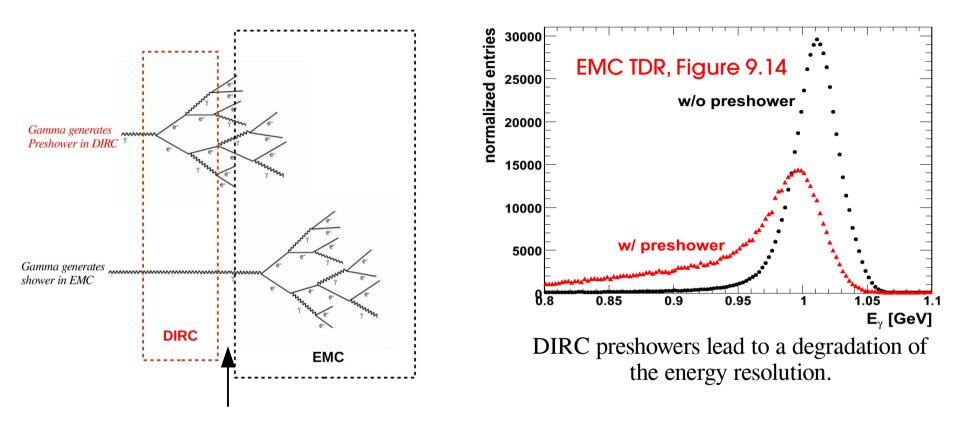
• In Panda, we have a SciTil in between DIRC and EMC, which has low material budget, insensitive to gamma, but has a high efficiency to charged particles. In a study for BaBar experiment, it was shown that, by detecting preshower by DIRC itself, 50% of the converted gamma can be recovered. But in our case, separate detector would discover conversion with full efficiency and enhance the energy resolution.
