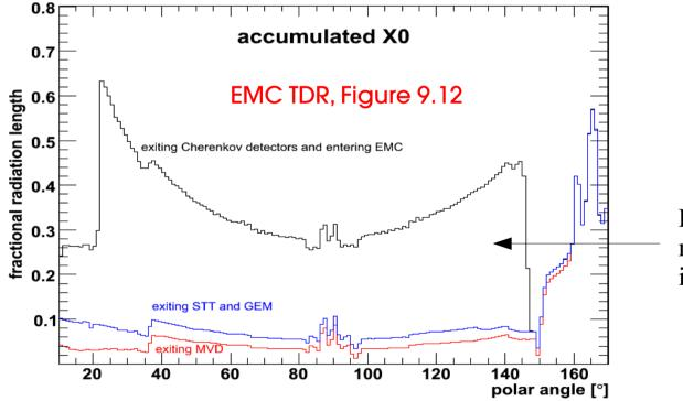
DIRC detector contributes most to the material budget in front of the EMC.
