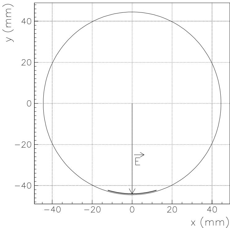
A 0.1 mm thin and 30 mm wide isolating  $Al_2O_3$  layer can be deposited at the bottom of the beam pipe using plasma spraying. On top of the isolating layer a 25 mm wide highly resistive thick film coating with a few 10  $\mu m$  thickness is applied. The highly resistive coating on top of the dielectric can be realized using commercially available thick film pastes from Heraeus. Reference: Fritz Caspers (CERN)
