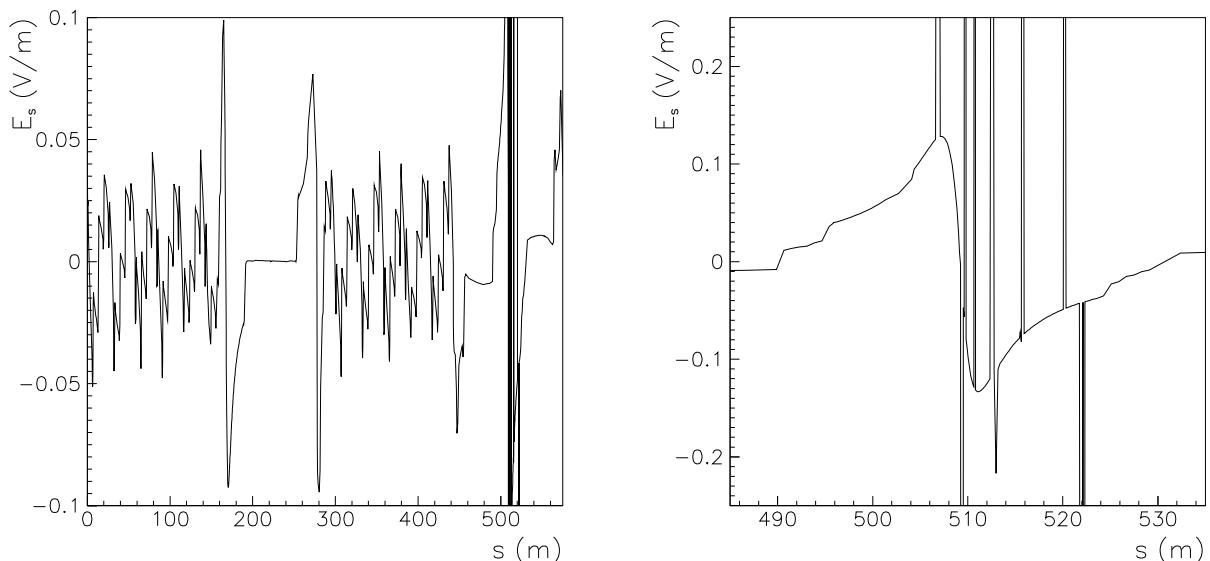
Longitudinal electric field component  $E_s$  of the antiproton beam assuming the standard optics,  $L_1 = 0.9C$ ,  $p_{\bar{p}} = 15$  GeV/c and  $N_{\bar{p}} = 1.0 \cdot 10^{11}$ .
