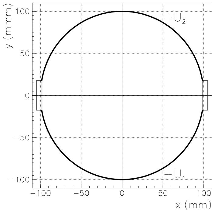
Neutralization electrodes at entrance and exit of EC as used at LEAR: Instead of extracting the ions which are produced by ionization of the residual gas in the EC, the ions are reflected and stored in the EC.
