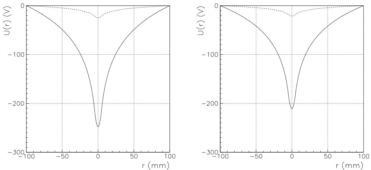
Space charge potential  $U(r)$  of the electron beam ( $I_e = 1.0 \text{ A}$ ,  $a = 5 \text{ mm}$ ,  $r_c = 100 \text{ mm}$ ). Full line: Beam neutralization  $\eta = 0.0$ . Dashed line: Beam neutralization  $\eta = 0.9$ . Left: Nominal kinetic energy 0.45 MeV. Right: Nominal kinetic energy 4.5 MeV.
