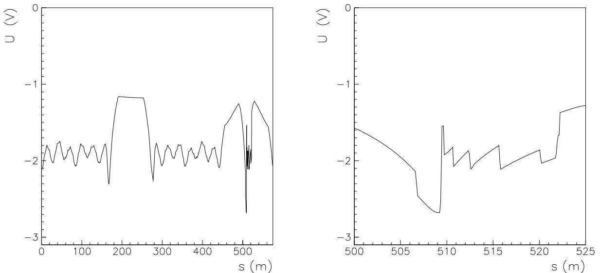
Central beam potential  $U(s)$  assuming the standard optics,  $L_1 = 0.9C$ ,  $p_{\bar{p}} = 15 \text{ GeV}/c$ ,  $N_{\bar{p}} = 1.0 \cdot 10^{11}$  and  $\eta = 0$ .
