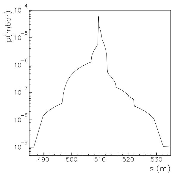
Vacuum pressure  $p(s)$  without NEG coating and heating jackets in the arcs.
