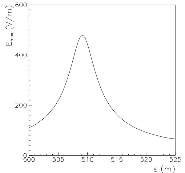
Upper limit  $E_{max}$  of the transverse electric field of the antiproton beam assuming the standard optics,  $L_1 = 0.9C$ ,  $p_{\bar{p}} = 15$  GeV/c and  $N_{\bar{p}} = 1.0 \cdot 10^{11}$ .
