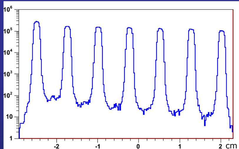
$\sigma_z \sim 200 \mu\text{m}$  along beam axis
