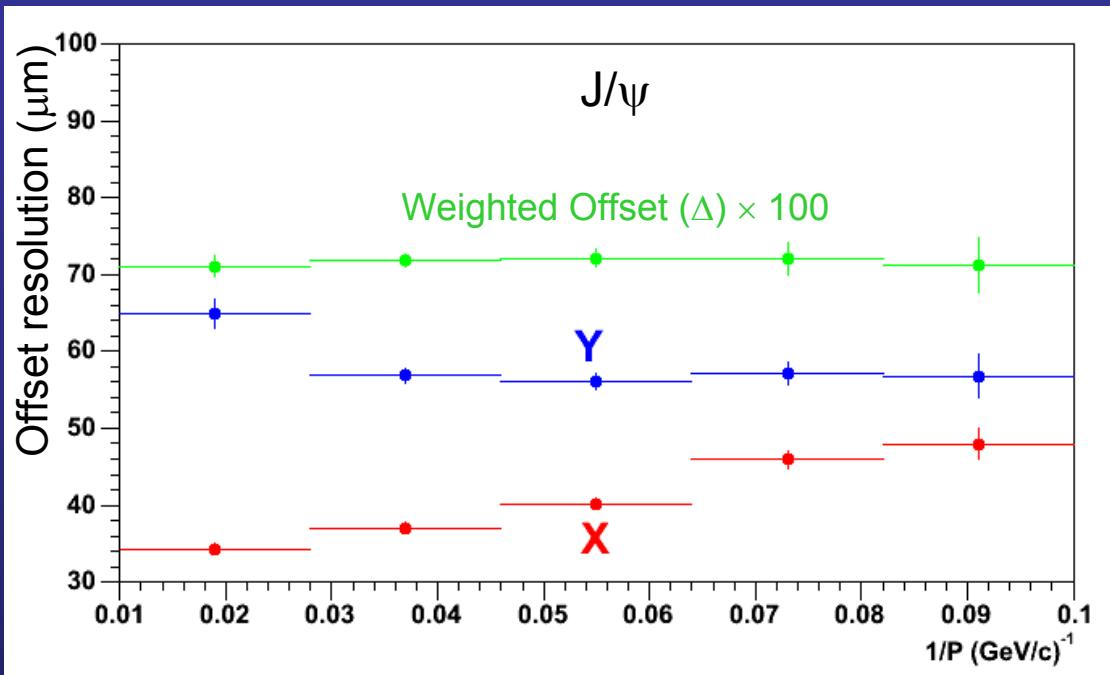
Resolution of the impact parameter of the track at the vertex (offset)
